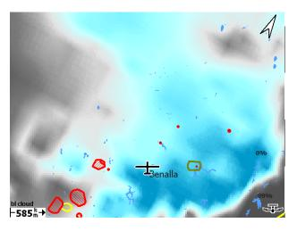
Sfc temp: The temperature at a height of 2 m above ground level. This can be compared to observed surface temperatures as an indication of model simulation accuracy; e.g. if observed surface temperatures are significantly below those forecast, then soaring conditions will be poorer than forecast.
