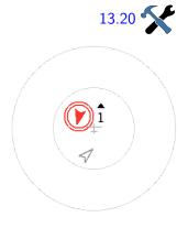
To remedy this situation, when FLARM traffic is received, XCSoar shows a small radar-style view of the FLARM traffic from the perspective of the aircraft. The FLARM traffic is displayed in identical style, except that the threatening traffic is emphasized with one or two red circles around the arrow head icon. The display corner used for the small radar view can be configured.
